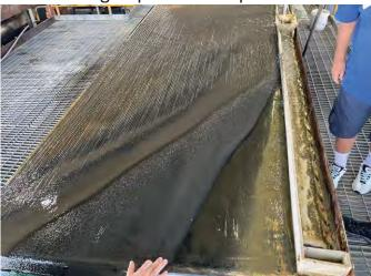
Separating tungsten using water & gravity
